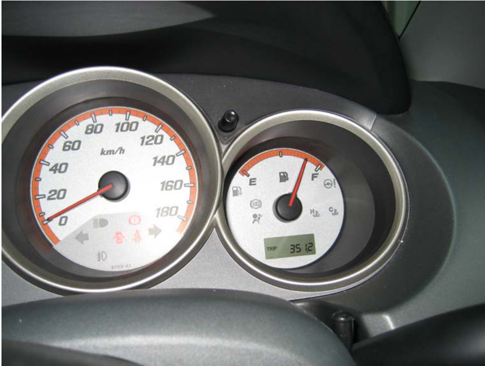
Tampered fuel gauge reading showed a three-quarter tank full of petrol
