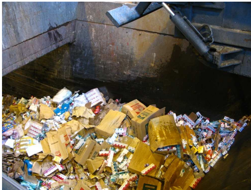
At the Tuas South Incineration Plant, the contraband cigarettes are off-loaded from the dump truck into the crusher pit where they are crushed before being incinerated.
